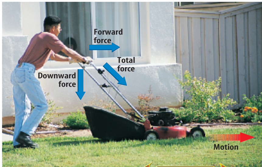
Figure 3 When you exert a force at an angle, only part of your force does work—the part that is in the same direction as the motion of the object.
