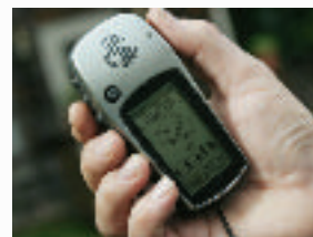
A modern GPS receiver uses a system of satellites to determine its position on Earth's surface.
