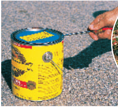
Figure 18 A lever is classified according to the locations of the input force, output force, and fulcrum.
