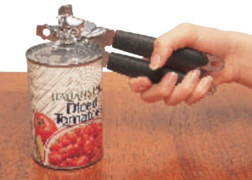
Figure 16 The can opener changes the small force of your hand on the handles to a large force on the blade that cuts into the can.
